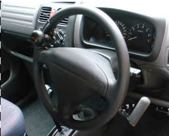
An adapted vehicle with steering ball and hand controls
